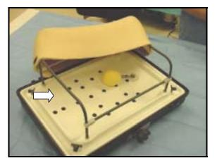
5. Fasten the crocodile clamp to the suction cup. Attach crocodile clamp to the balloon
